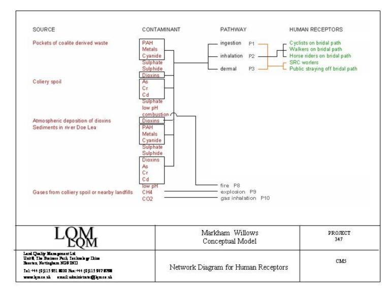
Figure 6.7 Example Conceptual Model Network Diagram for Human Receptors (Markham Willows Site - r3 2004)
