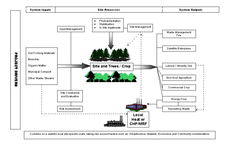
Figure 4.4 Phytoremediation and biomass concept based on SRC Part 1: inputs and outputs (Bardos et al. 2001)
