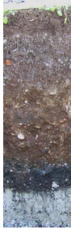
Technosol Constructed soil
